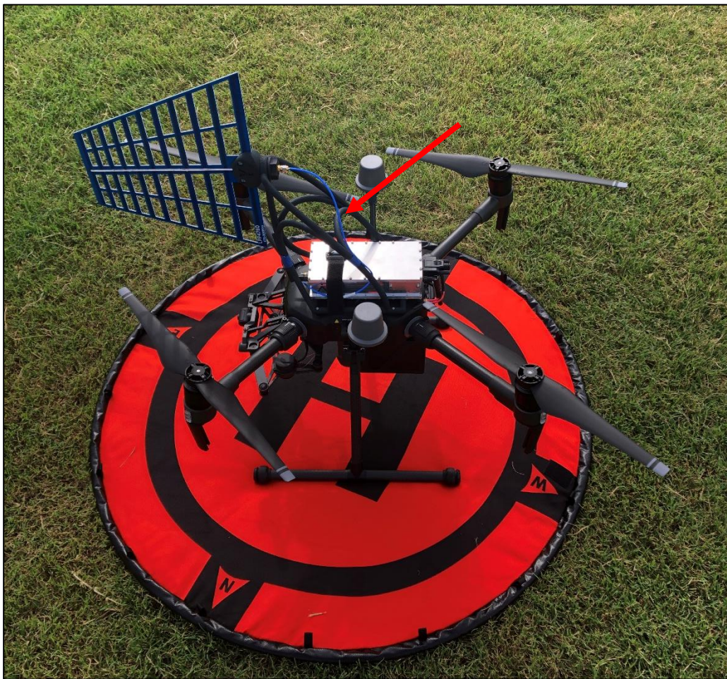
Suggested Rear Wifi Antenna Installation
