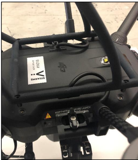
Align Antenna Frame with M200 mounting holes
