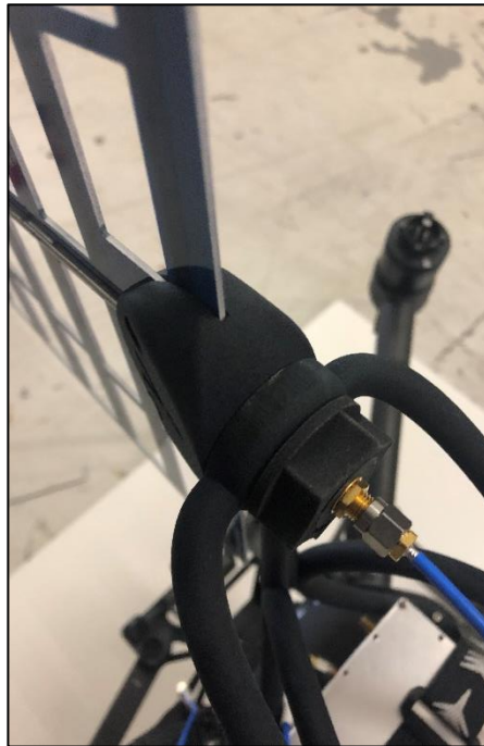
Attach RF Coax and Secure in place
