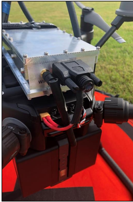
Suggested Rear Wifi Antenna Installation
