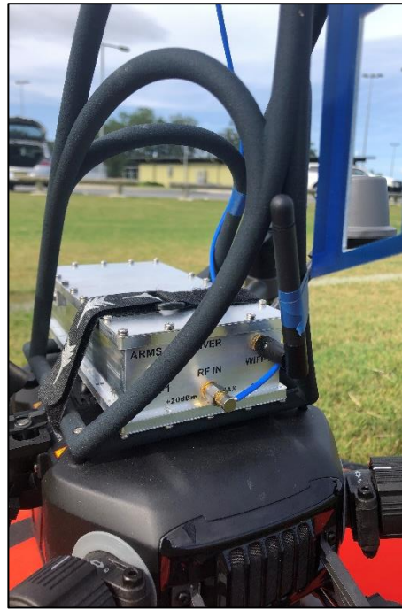
Suggested Front Wifi Antenna Installation
