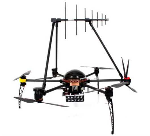
Fig. 2. ARMS Measurement Platform
