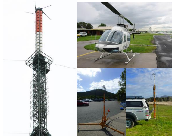
Fig. 1. Typical high-powered broadcast antenna systems (left) and Traditional measurement techniques (helicopter, portable mast and vehicle based mast).
