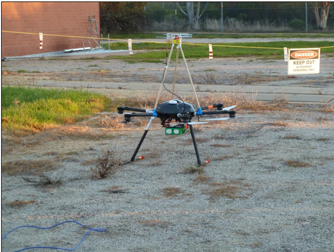
UHF TV Measurement System
