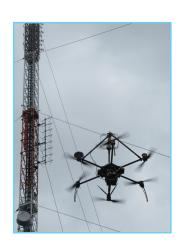
The system allows measurements of horizontal radiation patterns (HRP), vertical radiation patterns (VRP), effective radiated power (ERP), polarization discrimination and many other specific modulation parameters. Overall system uncertainties are in the order of 1-2 dB.
