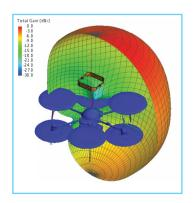
Each unit undergoes detailed electromagnetic modelling in order to assess the mounting position of the receive antenna on the UAV. This allows us to better understand the impact of the UAV on the receive measurements in order to improve overall system accuracies.
